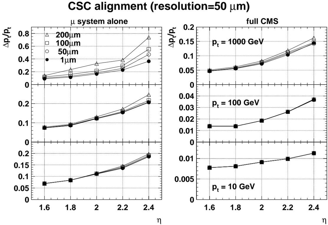
Figure 2: Momentum resolution for various values of alignment error assuming single layer  $\sigma = 50\mu\text{m}$ .
