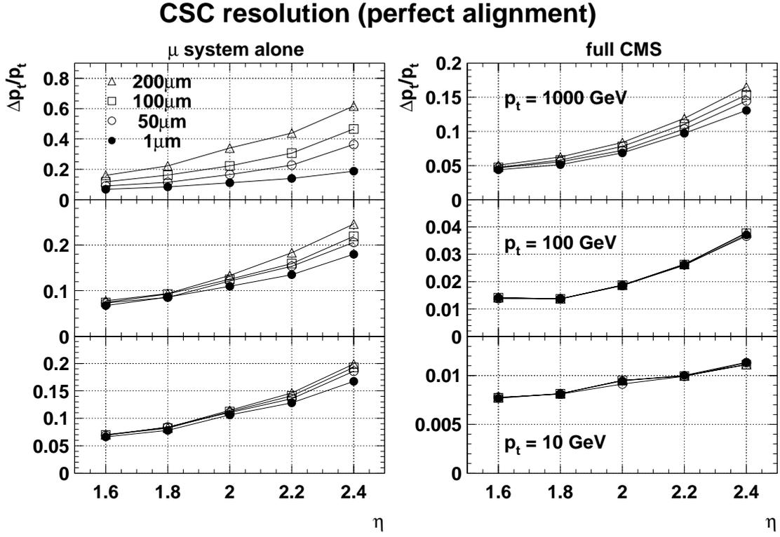
Figure 1: Momentum resolution for various single layer  $\sigma$  assuming perfect alignment.
