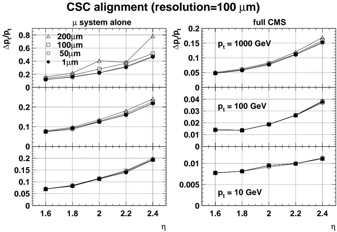
Figure 3: Momentum resolution for various values of alignment error assuming single layer  $\sigma = 100\mu\text{m}$ .
