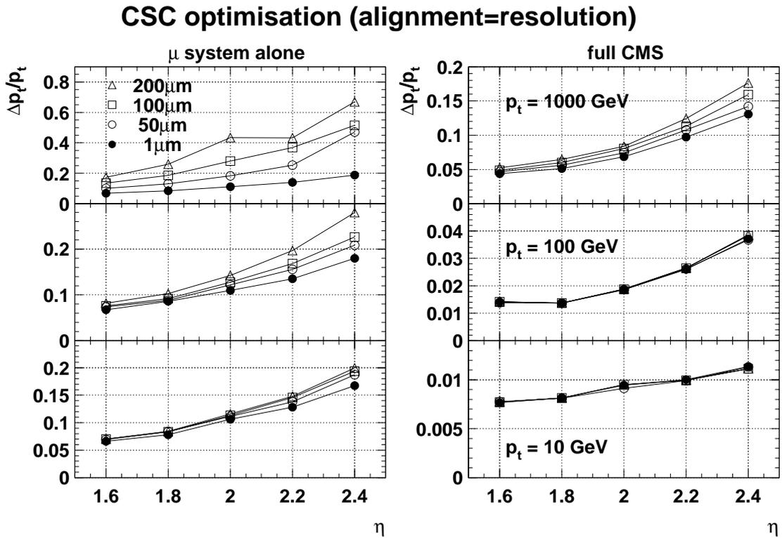
Figure 4: Momentum resolution for various values of alignment error and single layer  $\sigma$  assuming they are equal.
